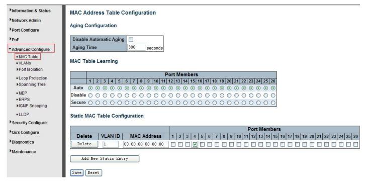
Figure 5-6 MAC Address Table Configuration Screen
