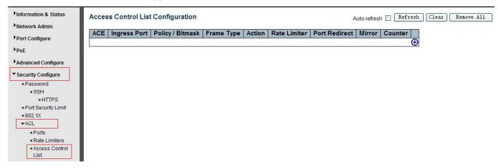
Figure 7-12 Access Control ListConfiguration Screen
