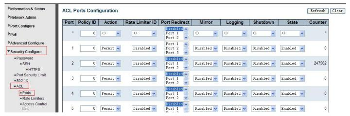
Figure 7-10 ACL Ports Configuration Screen
