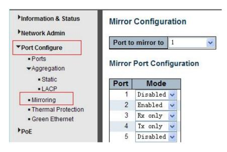
Figure 3-4Mirror Configuration Screen
