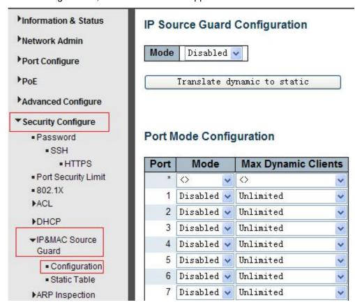
Figure 7-4 IP&MAC Guard- Port Configuration Screen
