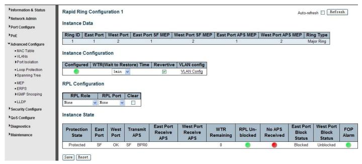
Figure 5-9EPRS Ring Configuration
