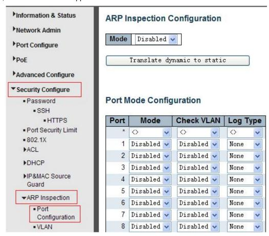
Figure 7-6 ARP Inspection Port Configuration Screen
