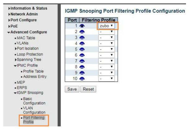
Figure 5-5-3 Port Filtering Profile Setting
