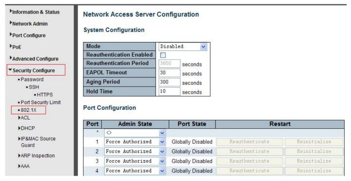
Figure 7-2 802.1XConfiguration Screen
