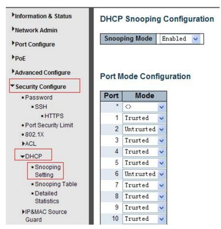
Figure 7-3DHCP Snooping Configuration Screen
