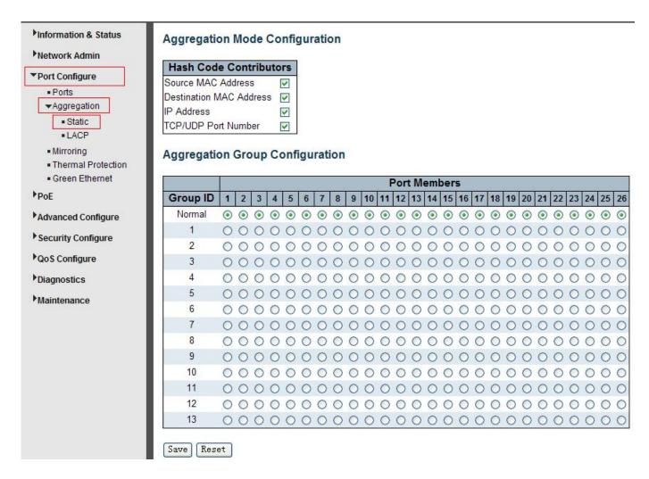
Figure 3-2Port Static Aggregation Configuration Screen
