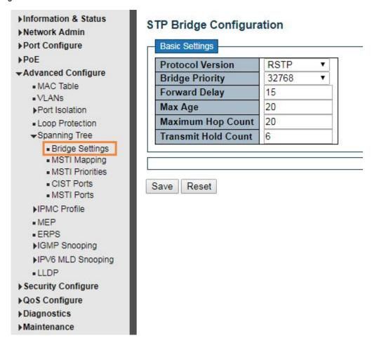
Figure 5-4 Spanning Tree Configuration Screen
