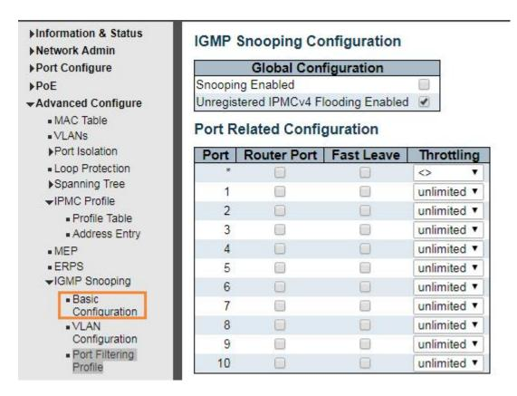
Figure 5-7 IGMP Snooping Basic Configuration
