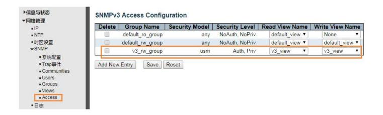
Figure 2-4-6 SNMPv3 Access Load Setting
