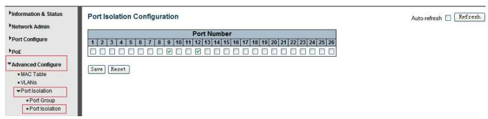
Figure 5-3 Port Isolation Configuration Screen
