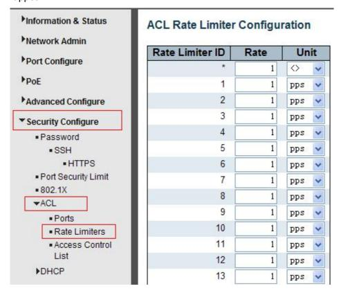
Figure 7-11 ACL Rate Limiters Configuration Screen
