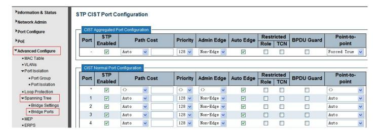
Figure 5-5 STPConfiguration Screen
