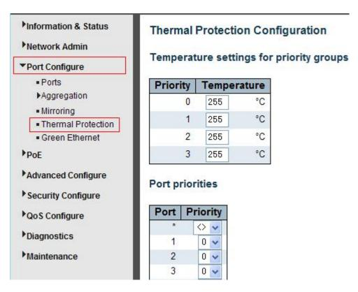
Figure 3-5Thermal Protection Configuration Screen
