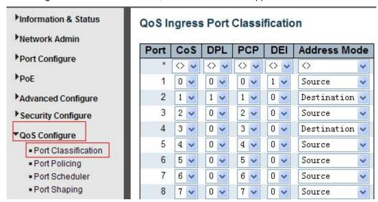
Figure 6-1 Port ClassificationConfiguration Screen
