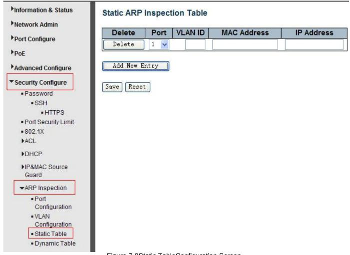
Figure 7-9Static TableConfiguration Screen
